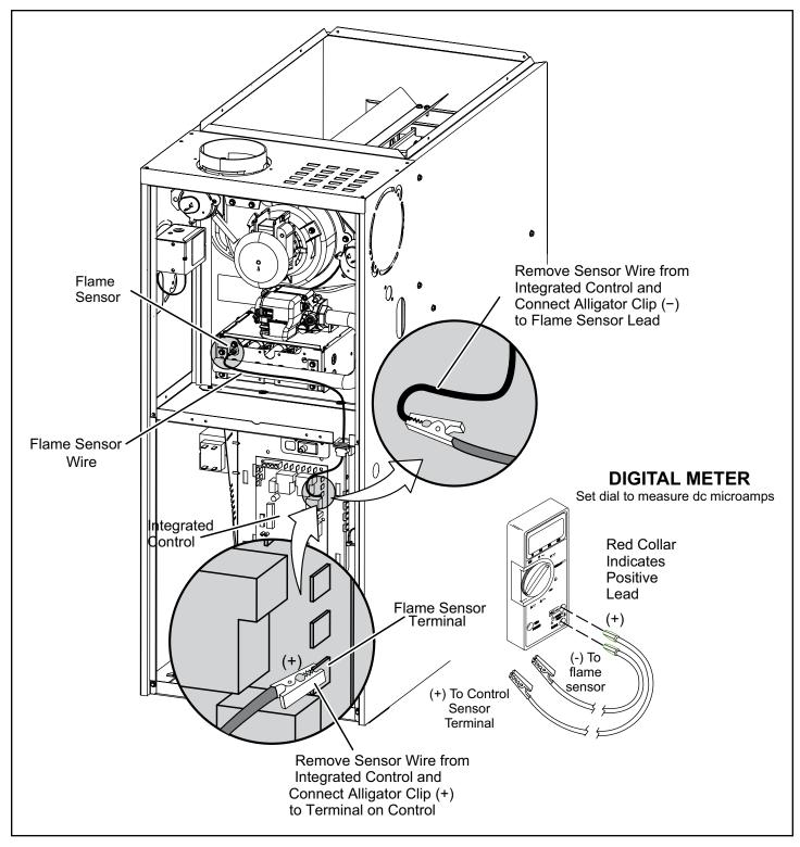
Figure 8. Measuring Flame Signal
