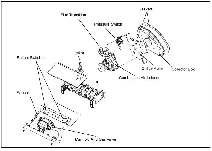
Figure 6. Heating Components
