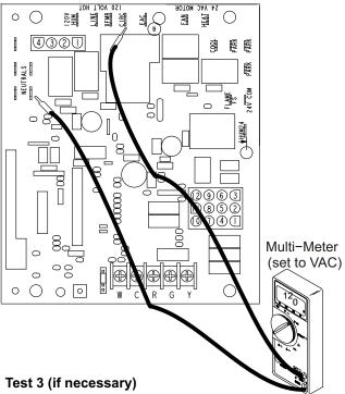
Check for 120 volts across terminals "CIRC" and "Neutrals" on the integrated control. If voltage is present, problem is with the harness. If voltage is not present problem may be may be with the integrated control.
