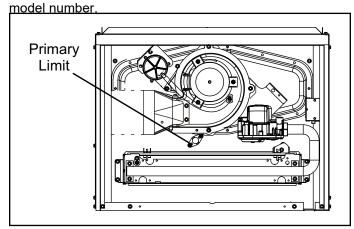
Figure 7. Primary Limit Under Combustion Air Inducer
