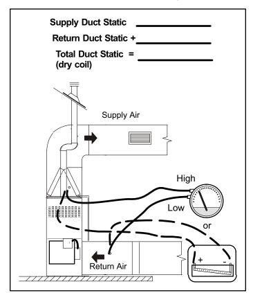
Figure 21. External Static Pressure
