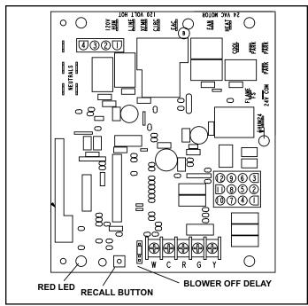
Figure 3. Integrated Control (Automatic Hot Surface Ignition System)
