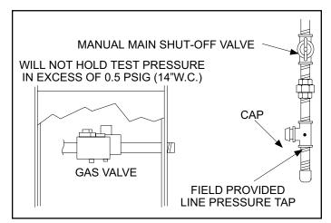
Figure 18. Gas Piping Test Procedure
