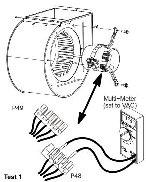
Turn on power to unit. Check for 120 volts across terminals "L" and "N" on input plug P48. If voltage is present continue to test 2. If voltage is not present, problem may be upstream of plug P48. Proceed to test 3.
